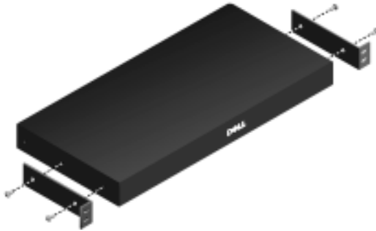
Figure 2-1. Console Switch Horizontal Installation
